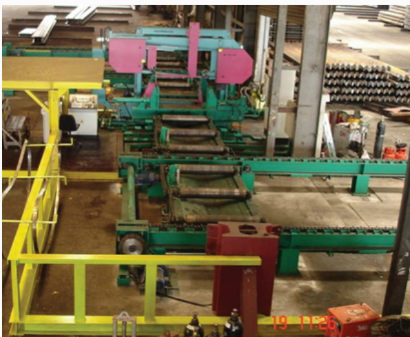
Heavy automatic chain transfer system
